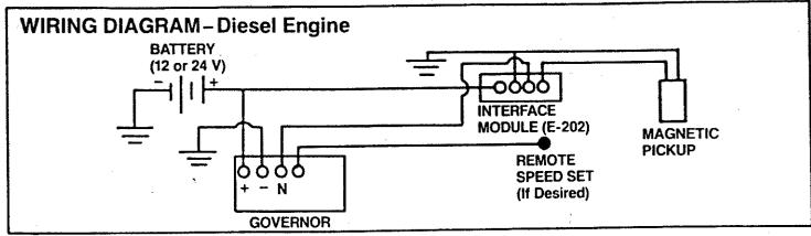
A properly functioning engine electrical system will run 13.5-14.5 VDC when the engine is running. Lower voltages can reduce governor output force and crispness of operation.
