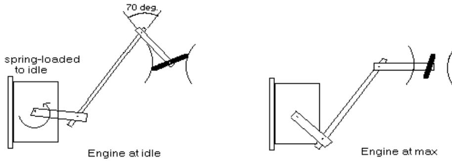
The needed **travel** of the carburetor determines how far out on the Actuator arm the rod is to be attached. In most cases, the carb should be moved from closed to about 10 degrees from full open as the actuator is moved from min to max. **THEN, ALTER THE LENGTH OF THE ROD SLIGHTLY (PERHAPS .030"), SO THAT THE ACTUATOR IS JUST OFF ITS INTERNAL STOP, AND IS PULLING THE BUTTERFLY AGAINST ITS STOP.** This insures that the carb can fully close to idle on load dumps, minimizing overspeeds.
